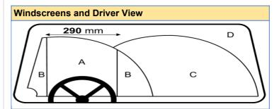
NO phone / sat-nav / dashcam placed in swept area ABCZone A: excludes damage, stickers or mounted items > 10mmZone B: excludes damage, stickers or mounted items > 40mmZone C: excludes damage, stickers or mounted items > 40mmRC86815Driver of motor vehicle not in position to have£100/3ptsfull view of road aheadRC86036Use motor vehicle when glass not maintained£50/0ptsto afford the driver unobscured vision
