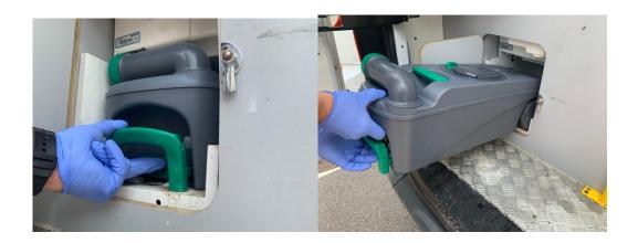
Gently lift up the locking button and the cassette can then be pulled out. It has an extendable handle and can be pulled on its wheels to a toilet.
