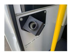
The water inlet point is by the crew door. Unscrew the cap and fill the tank with water – using a hose will save a lot of time. This is the water that will go through the sink taps and flush the toilet. Keep an eye on the water light to know when the tank is full.
