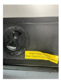
Under the table in the crew area is the water valve. Before attempting to fill the water tank you must ensure the valve is closed or the water will leak straight out! Unscrew the cap to locate the valve.
