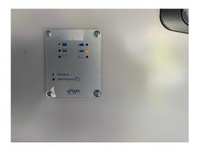
The left column shows the battery level. The right is the water level. When filling the water tank keep an eye on this light as it will go to green when it has enough water inside and will prevent you overfilling it.
