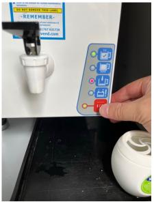
To use the hot water urn – fill it from the top by unscrewing the lid – do not overfill. Press the red power button to turn it on. If the battery light comes on there is an error – drain the urn and do not use. The next 2 lights indicate there is not enough water and then that it is heating. The top light means the water is hot enough to use. When the van is returned please drain the urn before driving to prevent leaks and the crew area flooding!
