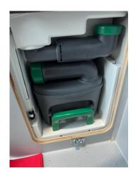
In the storage area of the van, you will find the hatch to access the clean water flush and the waste cassette. THE TOP FUNNEL IS FOR FRESH WATER!!
