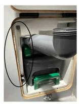
Gently pull the top spout towards you and remove the lid. Add the contents of the pink bottle. Carefully pour water into it, there is a clear plastic hose to the left and this is the gauge as to how full the tank is. When you see the water level ¾ to the top of this tube the tank has enough water in it.
