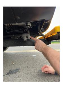
Finally, when you return the van you must empty the waste water tank (this is waste from the sink don't worry!) It is located under the rear step, simply open the tap and the wastewater can drain away.
