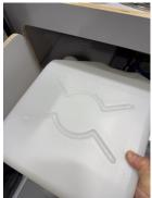
Under the sink in the kitchen area you will find the freshwater tank. Empty two whole water containers into this CAREFULLY! If you spill any clean it up. Do not over tighten the tank lid – a vacuum is created inside and if it is too tight it will not come off.
