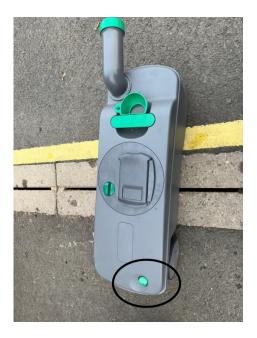
Gently rotate the spout out and the waste can be emptied into a toilet. You will need to hold the button down circled in this picture.
