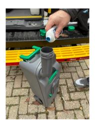
Rotate the spout up and unscrew the lid. Empty the blue chemical into the cassette. Replace the lid and gently slide the cassette back into place.
